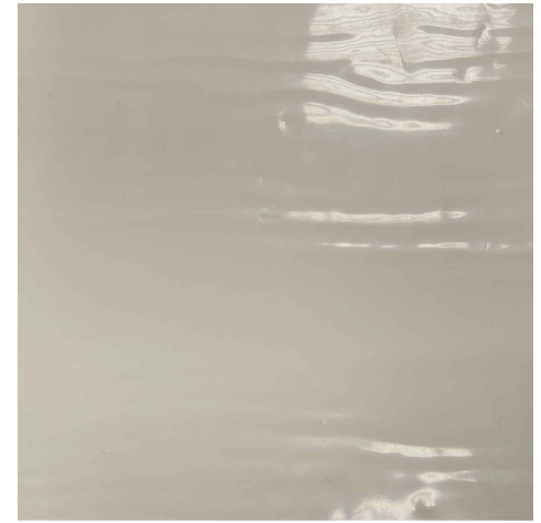
White HDPE to face installer. (THIS SIDE UP)
