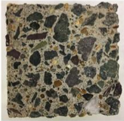
Figure 3. OPC after sulphuric acid test showing deterioration.
