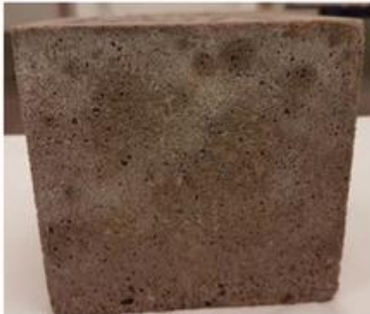
Figure 4. Cemfree low-carbon cement after sulphuric acid test, showing a lot less deterioration.
